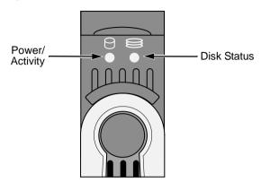
Figure 3. VTrak M500f/i/p Drive Carrier LEDs.
